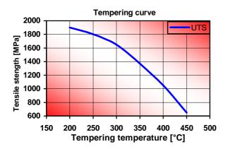
Tempering curve of a sample which has been austenitised at 830 °C.
