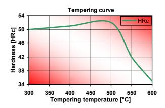
Tempering curve of a sample which has been austenitised at 980 °C.
