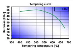
Tempering curve of a sample which has been austenitised at 1020 °C. The diagram shows values obtained after the second temper.
