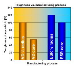
Thanks to the ESR process, Eskylos® 2344 satisfies the most difficult requirements in terms of toughness and suitability to polishing. It is suitable for the manufacture of moulds subjected to mirror polishing and to high mechanical stress.
