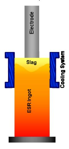
The result is homogeneous and isotropic steel.
