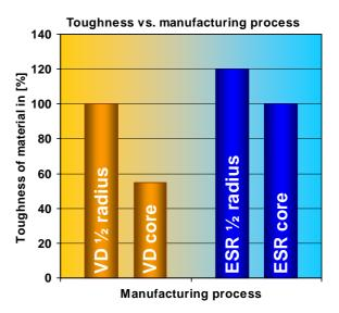
Thanks to the ESR process, EskyLos<sup>®</sup> 2343 satisfies the most difficult requirements in terms of toughness and suitability to polishing. It is suitable for the manufacture of moulds subjected to mirror polishing and to high mechanical stress.
