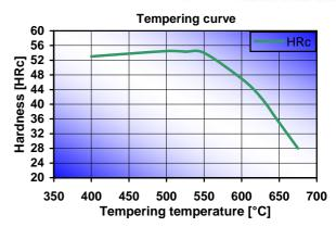
Tempering curve of a sample which has been austenitised at 980 °C. The diagram shows values obtained after the second temper.
